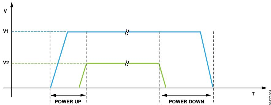
Figure 1. Typical Sequencing Requirement for Power-Up and Power-Down
