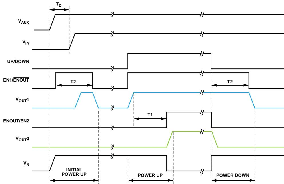
Figure 3. Circuit Timing Diagram
